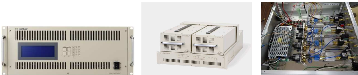
Figure 1. RF Direct sampler OCTAD manufactured by Elecs industry.
