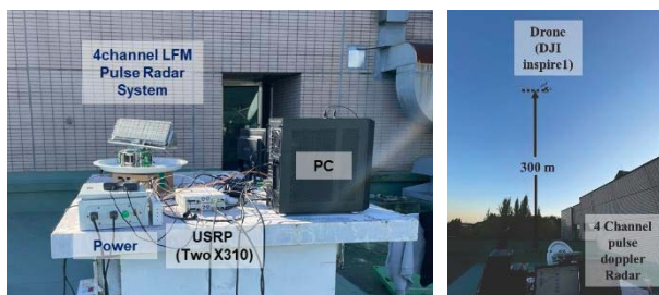
Figure 1. Pulse Doppler radar structure and experimental setup
