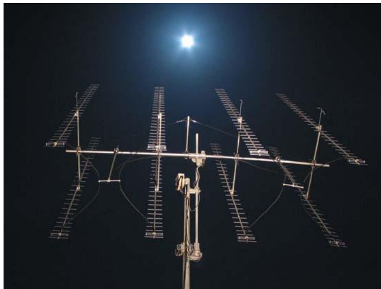
Figure 1. EME system: Array of eight high-gain Yagi antennas in the 420-440 MHz
