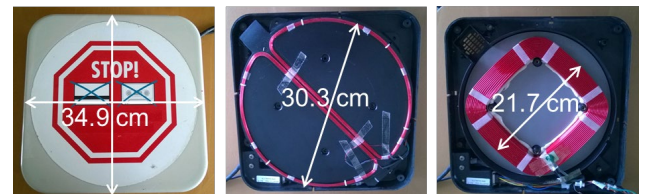
Figure 1. Investigated AM-EAS deactivator. Left: top view of the fully assembled device; center: removed top cover shows detection coil; right: removed detection coil shows deactivation coil.
