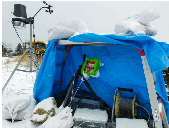
Figure 1. Long-range MIMO type GB-SAR observation during snow in Sendai, Japan.
