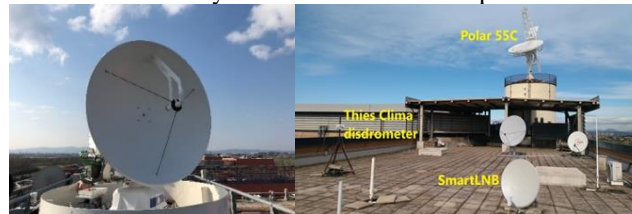
Figure 1: (left) Weather radar WR25XP in Florence; (right) set-up at ISAC-CNR during NEFOCAST.
