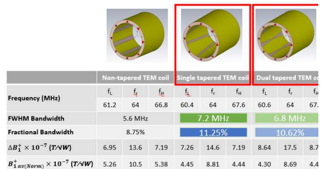
Figure 1. Comparison of performances of traditional TEM, and single tapered and double tapered TEM [5]
