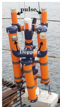
Figure 4. Acoustic wave gauge before the installation.
