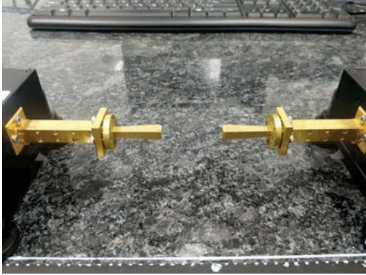
Figure 2. Pyramidal horn antennas as transmitter and receiver
