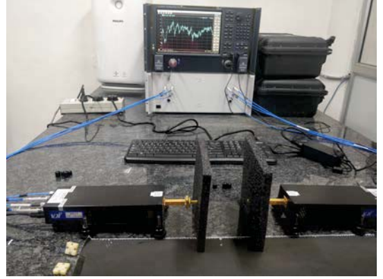
Figure 4: Radiating near field measurement setup
