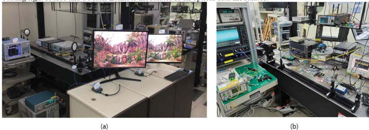
Figure 1. Photograph of experimental setup for THz wireless link (a) with 25 Gbps data rate using directly modulated DFB-LDs as a beating light source and a data modulator, (b) with 100 Gbps data rate using free running lasers as beating light sources and an Mach-Zehnder modulator as an optical data modulator.
