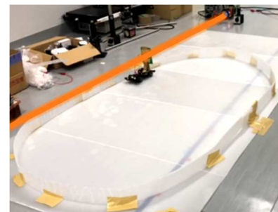
Figure 3. Dynamic power transmission to a hobby car by OWPT. The line shows the beam position.
