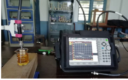
Figure 8. Experimental set up for the measurement of permittivity of liquid samples.
