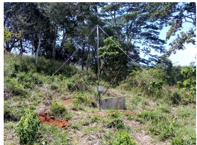
Figure 1: ELF/VLF receiver in Sri Lanka. It is in the Hantana mountain range and managed by University of Peradeniya.
