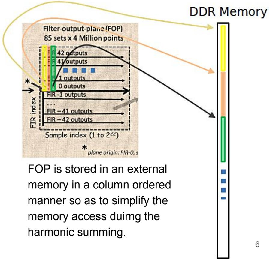
FOP is stored in an external memory in a column ordered manner so as to simplify the memory access during the harmonic summing.
