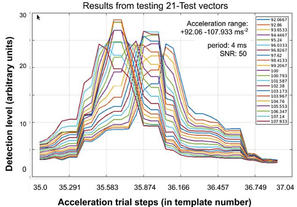
Overlay of 21 result profiles from the prototype presented here. Acceleration cases between 92 and 108 m/s/s, period 4 ms and SNR 50 considered. The detections show peak values in the profiles and they shift (as expected) from the left to the right with accelerations changing from 107.9 to 92 m/s/s.
