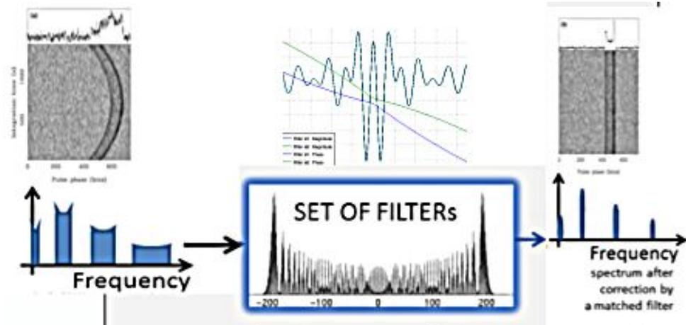
Conjugate coefficients are used in the matched filtering.
