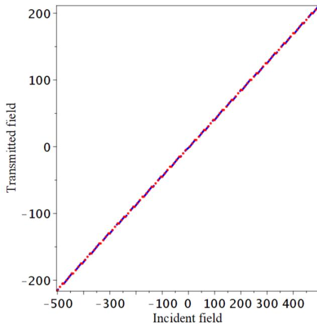
Рис. .3: Amplitude of the transmitted field  $F_T$  vs amplitude of the incident field  $F_I$  in the linear ( $\alpha = 0$ , blue) and nonlinear (red) cases. The values of parameters are  $\gamma = 1.15$ ,  $k_0^2 = 1$ ,  $r_0 = 2$ ,  $r = 4$ ,  $\varepsilon^2 = 4$ ,  $\alpha = 10^{-5}$ .
