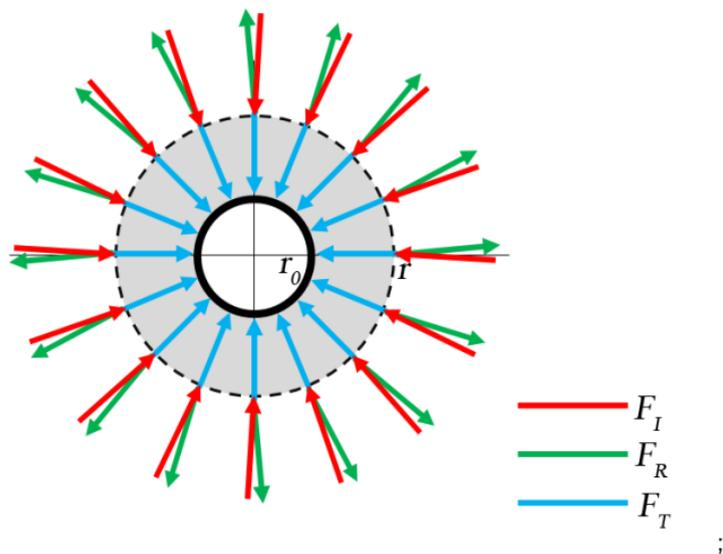
Рис. .1: Waveguide  $\Sigma$ , where  $r_0$  and  $r$  are the radii of the internal (perfectly conducting) and external (dielectric) cylinders, respectively.
