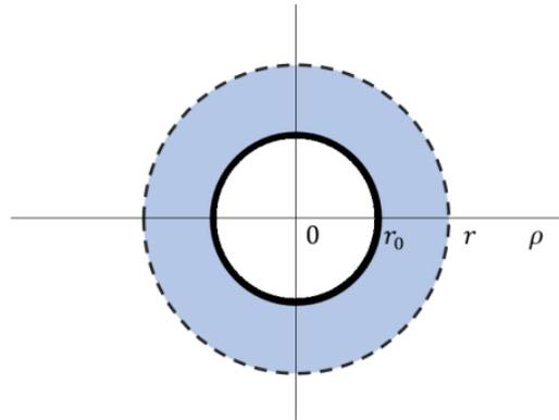
Рис. .1: Goubau line; a single wire conductor coated with dielectric material.
