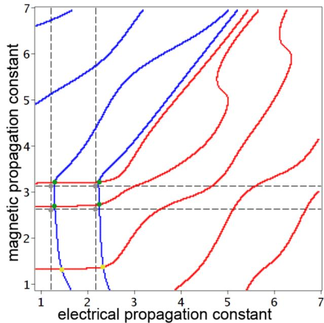
Рис. 3:  $\varepsilon = \varepsilon_c + \rho$ ;  $\varepsilon_c = 11.7$  (Si);  $r_0 = 2$  mm and  $r = 4.2$  mm,  $C_E = C_M = 1$ ;  $\omega_E = 30$  GHz,  $\omega_M = 40$  GHz;  $\alpha = 1$  mmV<sup>-1</sup>.
