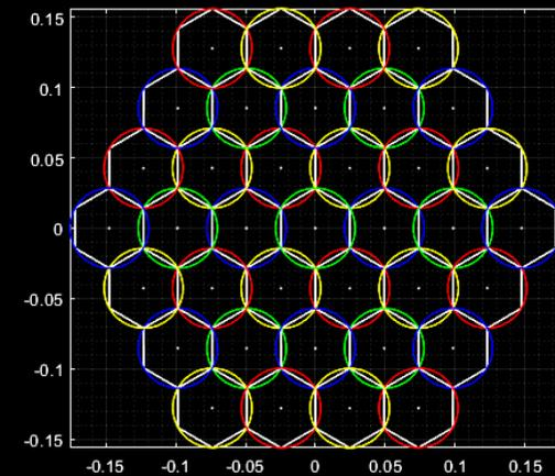
Uniform Cell pattern with 4cell reuse scheme
