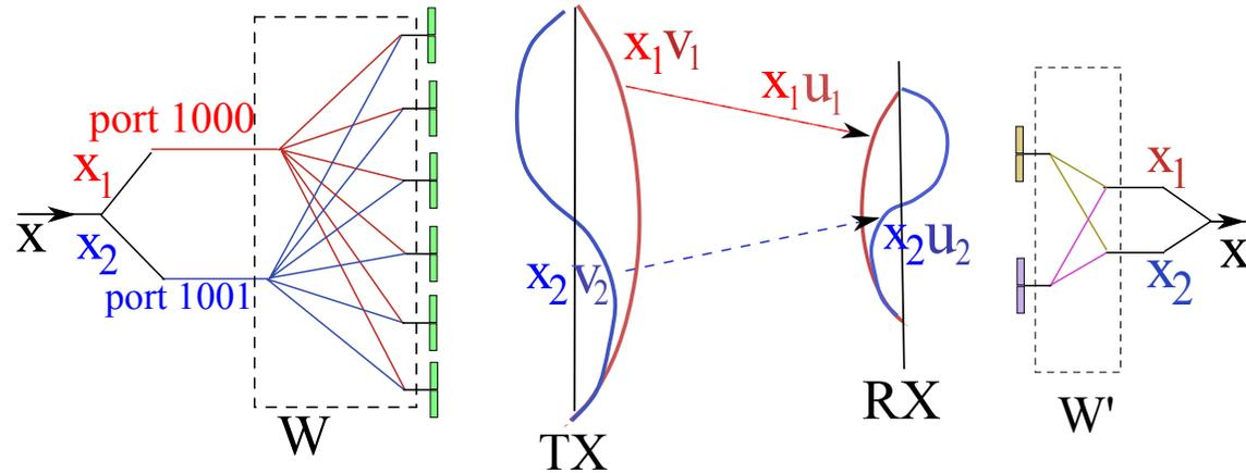
In case of planar radiating surfaces the SNDF is almost equal to 4 times to the electrical area of the radiating surface, i.e.  $4 A/\lambda^2$ , wherein  $A$  is the area and  $\lambda$  is the wavelength
