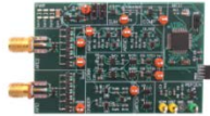
Figure 1—Our Prototype integrates both \mu mo and \mu code in a single design. It can operate using both RFID and TV transmissions.
