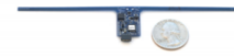
Fig. 1. The wireless identification and sensing platform (WISP) [8] is a programmable sensor platform based on RFID. It is wirelessly powered and uses backscatter modulation to relay sensor information to a RFID reader.
