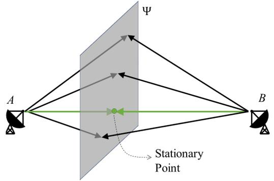
**Figure 2.** Illustration of stationary point identification approach. Among the ray pairs which emanate from  $A$  and  $B$ , those which are marked as green yield the path with shortest length. The intersection point of these rays with the surface  $\Psi$  is the stationary point.
