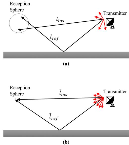
**Figure 1.** Illustration of the ray path length differences for a small/large number of ray launches and accordingly chosen reception sphere sizes. The errors are likely to be more drastic for  $l_{los}$  and  $l_{ref}$  than  $\tilde{l}_{los}$  and  $\tilde{l}_{ref}$
