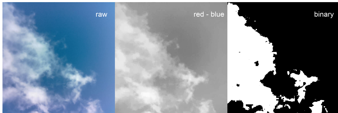
Figure 1. Sample cloud cover measurement from the SMA field test. The difference of the red and blue channels from a raw image is calculated, and pixels exceeding a threshold are logged as clouds.
