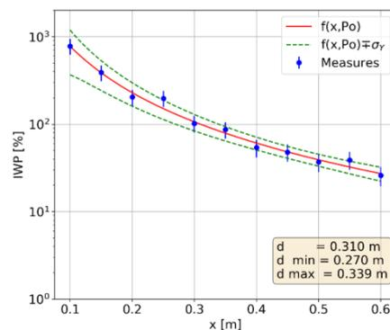
**Figure 1.** Interpolation of the weighted peak exposure index measured in the vicinity of an arc-welding device:  $d=31\text{cm}$  is the nominal respect distance,  $d_{\text{min}}=27\text{ cm}$  and  $d_{\text{max}}=33,9\text{ cm}$  are the values evaluated propagating the measurement uncertainty considering a coverage factor  $k=1$ .
