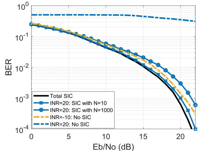
Figure 2. Comparison of the BER performance of the FDSM system with different SIC levels (total SIC, no SIC, SIC with 10 or 1000 test numbers)
