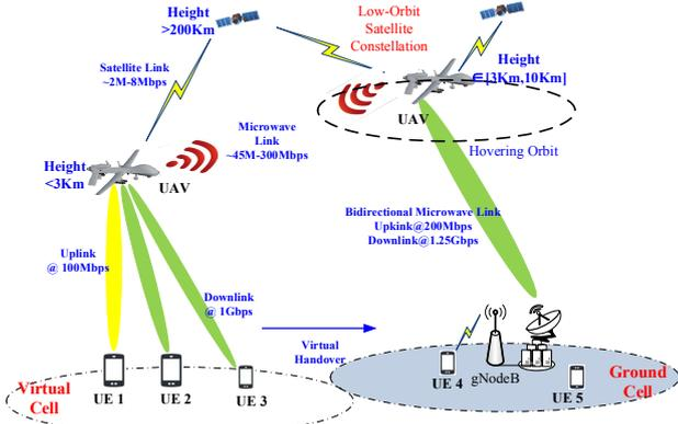
**Figure 1.** UAV 5G Network Architecture. Low Orbit Satellite and UAV served in different region.
