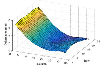
Figure 4. Deformation shape of the antenna.
