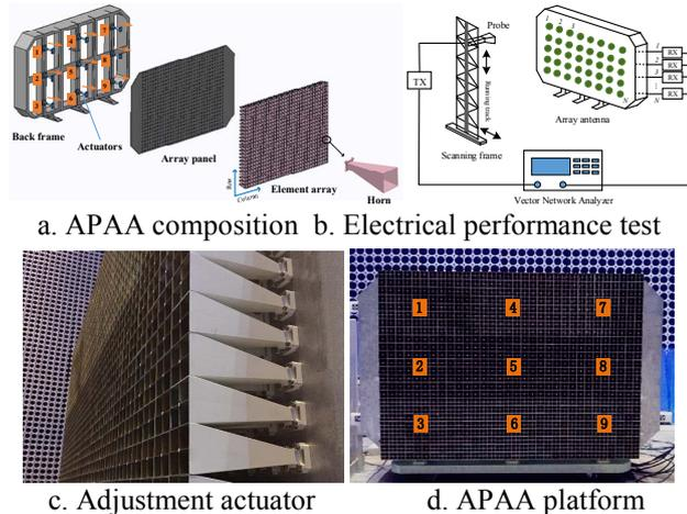
Figure 3. Architecture of APAA platform.
