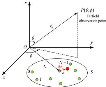
**Figure 2.** Array antenna elements in arbitrary distributed.
