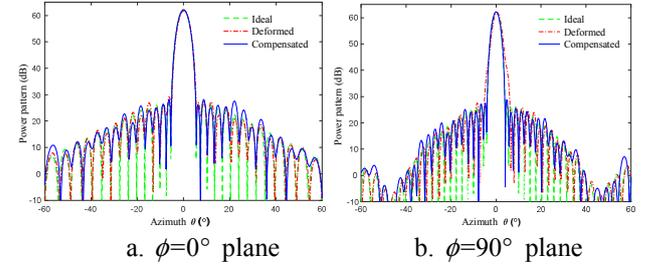
Figure 6. Performance before and after compensation.
