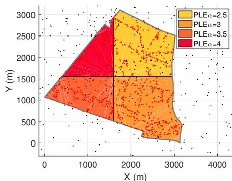
**Figure 2.** Block-based path loss model, different colors represent different regions covered by different PLE.
