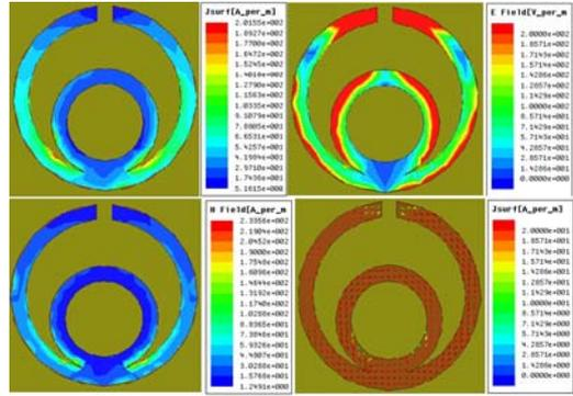
**Figure 5.** Microscopic properties of SSR: Magnitudes of Current, Electric field, Magnetic field and Current distribution with its phase
