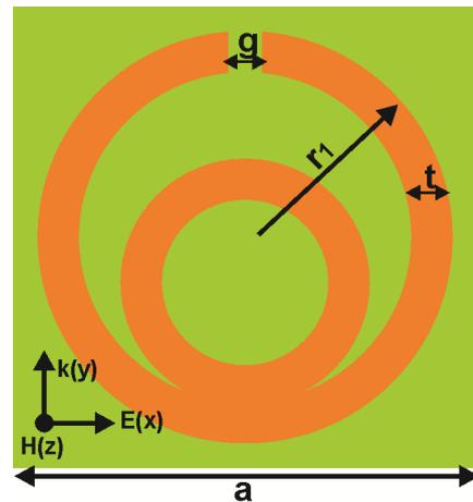
**Figure 1.** Structure of a unit cell with its dimensions and field vectors ( $r_1=12\text{mm}$ ,  $g=1\text{mm}$ ,  $t=2\text{mm}$ )
