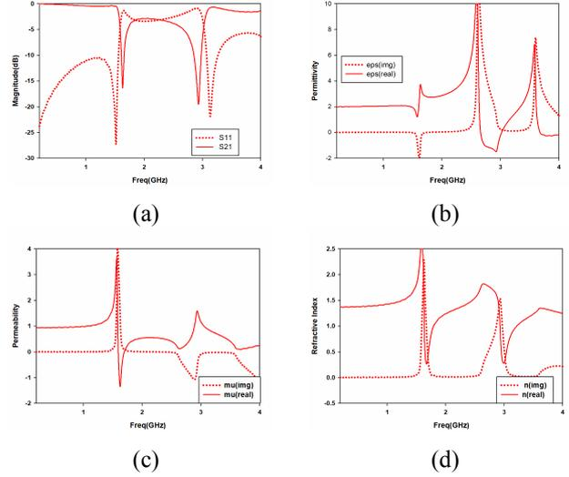
**Figure 4.** (a) Transmission and reflection coefficient (b) Permittivity (c) Permeability (d) Refractive Index
