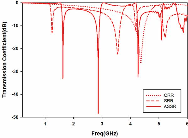
**Figure 3.** Simulated Transmission coefficients of (a)CRR (b)SRR (c)ASSR
