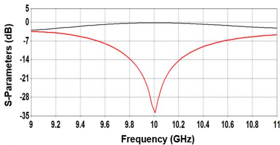
**Figure 5.** S-parameter of FC-75 in double disc RF window.
