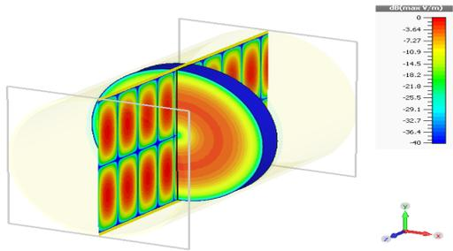
**Figure 3.** RF wave propagation and its absorption in FC-75 double disc RF window
