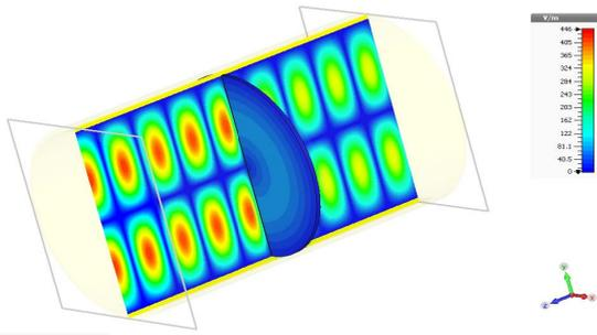
**Figure 2.** RF wave propagation and its absorption in EG double disc RF window
