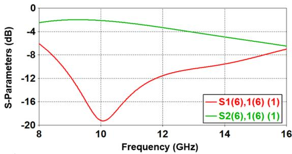
**Figure 4.** S-parameter of EG in double disc RF window.
