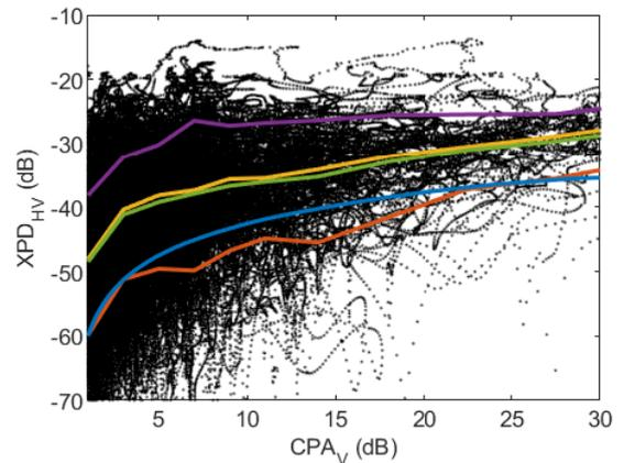
**Figure 5.** Scatterplot of  $XPD_{HV}$  and  $CPA_V$ , at 49.5 GHz. Red, yellow and purple curves are the 10, 50 and 90 percentiles of XPD conditioned to CPA values. The green curve is the mean. The cyan curve is the ITU-R P.618-13 model prediction.
