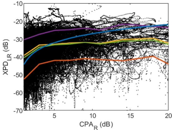
**Figure 3.** Scatterplot of  $XPD_{LR}$  and  $CPA_R$ , at 39.6 GHz. Red, yellow and purple curves are the 10, 50 and 90 percentiles of XPD conditioned to CPA values. The green curve is the mean. The cyan curve is the ITU-R P.618-13 model prediction.
