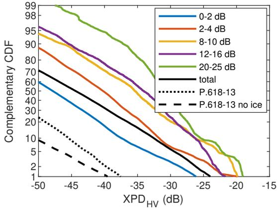
**Figure 6.** Gaussian integral chart of the XPD CCDFs at 49.5 GHz, not conditioned (black curve) and conditioned (coloured curves) to the selected CPA ranges. The dotted and dashed curves represent the ITU-R P.618-13 CCDF predictions, respectively including and neglecting the effect of the ice.
