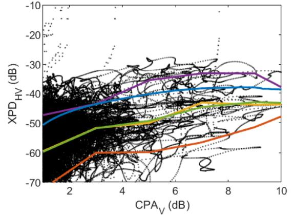
**Figure 1.** Scatterplot of  $XPD_{HV}$  and  $CPA_V$ , at 18.7 GHz. Red, yellow and purple curves are the 10, 50 and 90 percentiles of XPD conditioned to CPA values. The green curve is the mean. The cyan curve is the ITU-R P.618-13 model prediction.
