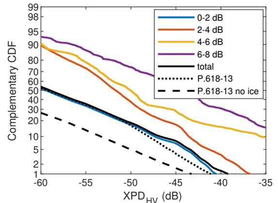
**Figure 2.** Gaussian integral chart of the XPD CCDFs at 18.7 GHz, not conditioned (black curve) and conditioned (coloured curves) to the selected CPA ranges. The dotted and dashed curves represent the ITU-R P.618-13 CCDF predictions, respectively including and neglecting the effect of the ice.
