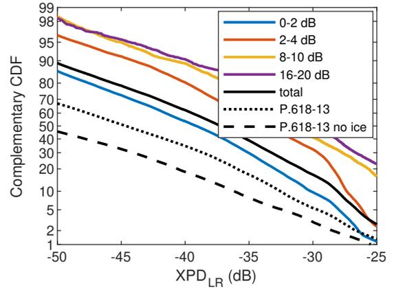
**Figure 4.** Gaussian integral chart of the XPD CCDFs at 39.6 GHz, not conditioned (black curve) and conditioned (coloured curves) to the selected CPA ranges. The dotted and dashed curves represent the ITU-R P.618-13 CCDF predictions, respectively including and neglecting the effect of the ice.
