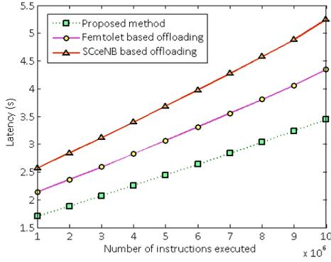
Figure 2. Latency in computation offloading
