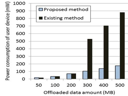
Figure 5. Power consumption of the user device during data offloading
