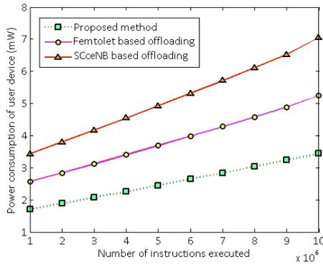
Figure 3. Power consumption of the user device during computation offloading
