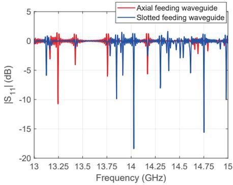
**Figure 5.**  $|S_{11}|$  for the launch configurations (a) and (b). The slotted waveguide launch excites a large number of modes inside the cavity with respect to the classical axial launch scheme.
