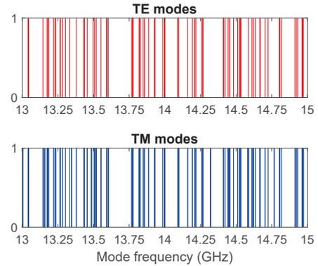
**Figure 4.** Bar plot of the TE and TM modes inside the cylindrical cavity in the frequency interval of [13;15] GHz.
