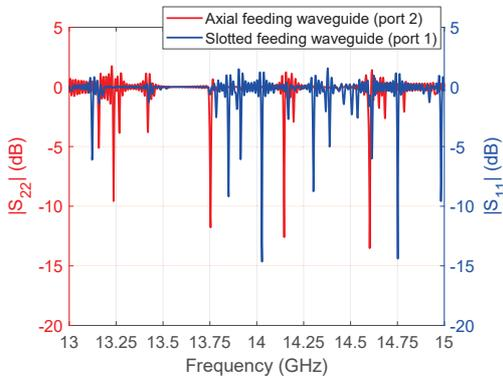
**Figure 6.**  $|S_{11}|$  and  $|S_{22}|$  for the launch configuration (c). The presence of both launch schemes do not alter the modal distribution inside the band of interest.
