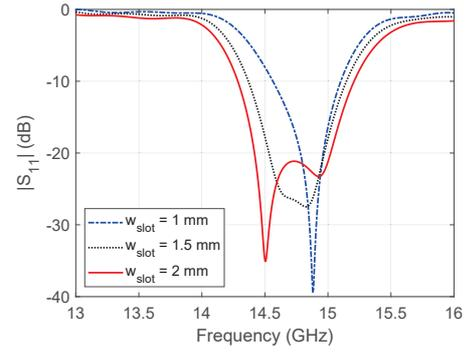
**Figure 3.**  $|S_{11}|$  vs. slot width  $w_{slot}$ : it can be seen that this parameter affects the impedance bandwidth.
