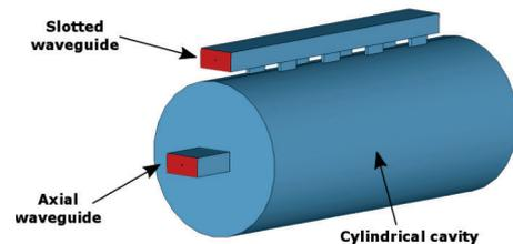
**Figure 1.** Simulated cylindrical chamber geometry with the axial and slotted waveguide launch structures.
