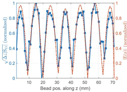
**Figure 7.** Field profile obtained with the bead-pull technique (blue marked curve) vs. simulated field profile extracted along the cavity axis for a length of 140 mm (red dot-dashed curve).
