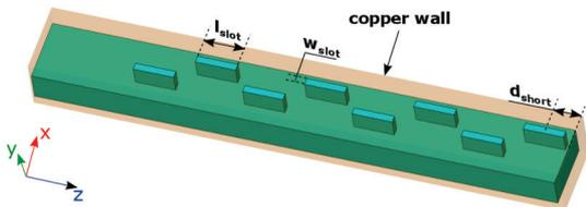
**Figure 2.** Slotted waveguide antenna model with its fundamental parameters: slot length  $l_{slot}$ , width  $w_{slot}$  and distance from the short circuit  $d_{short}$ . The air volume (blue object) and the copper enclosure (orange semitransparent object) are visible.
