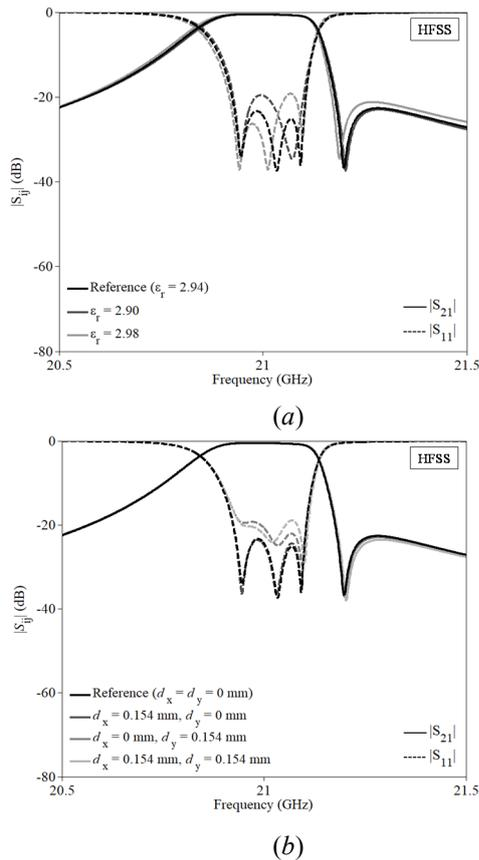
**Figure 4.** Robustness analysis against (a) dielectric constant variation using HFSS and (b) multilayer misalignment using HFSS.
