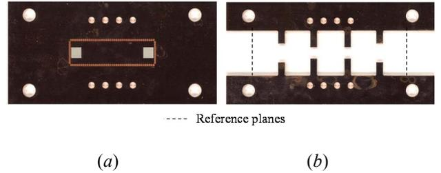
**Figure 5.** Photographs of (a) substrate 1 and (b) substrate 2 of the fabricated third-order with 1-3 cross-coupling AFSIW filter demonstrator. The dimensions of the fabricated filter are  $61.8 \times 31.15 \times 2.54$  mm<sup>3</sup>.
