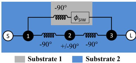
**Figure 2.** Coupling diagram, with source/load coupling, of the third-order AFSIW filter.
