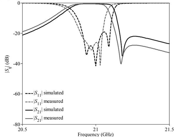
**Figure 6.** Simulated and measured S-parameters of the fabricated third-order 1-3 cross-coupled AFSIW filter demonstrator.
