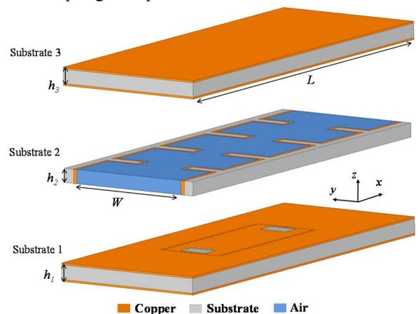
**Figure 1.** 3D view of the third-order in-line air wave with 1-3 cross-coupling AFSIW filter.
