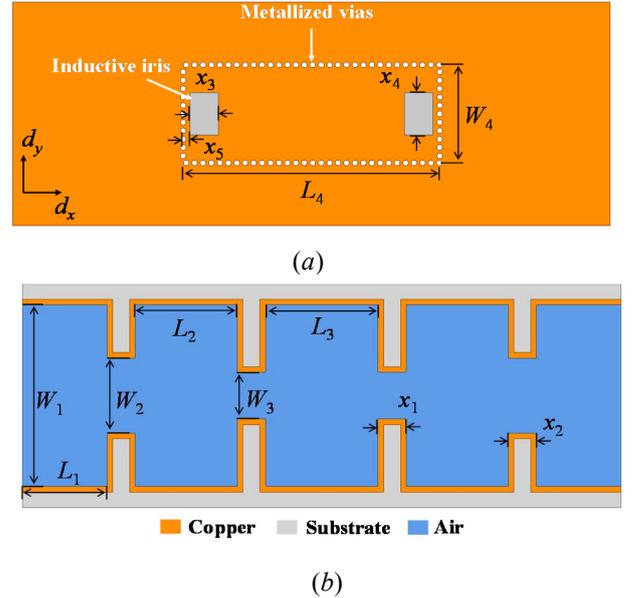
**Figure 3.** Top views of (a) substrate 1, implementing the secondary path with the 1-3 cross-coupling, and (b) substrate 2 implementing the primary path with the three resonators using high  $Q$ -factor propagation medium.
