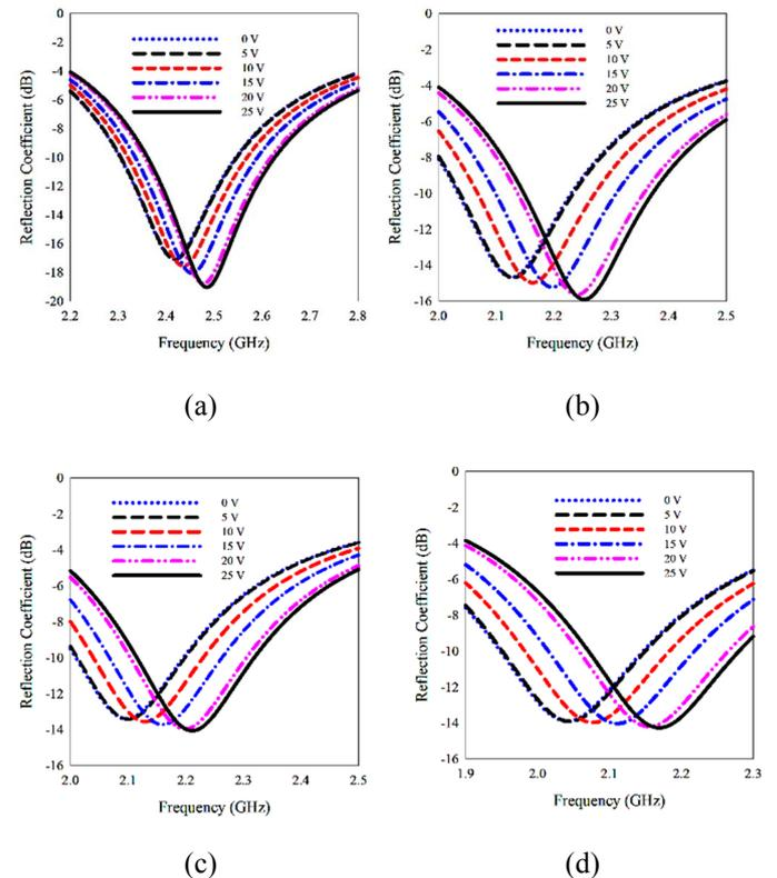
**Figure 4.** Simulation results of frequency switching (a) Enabling D1 and D2 (b) Activating D1-D4 (c) Enabling D1-D6 (d) Activating D1-D8.
