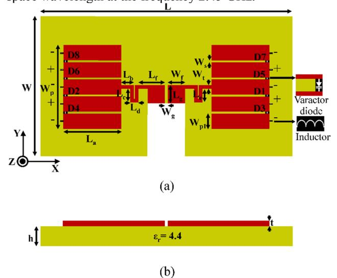
**Figure 1.** Geometry of the proposed dipole antenna ( $L=0.408 \lambda_0$ ,  $W=0.245 \lambda_0$ ,  $L_a=0.081 \lambda_0$ ,  $W_g=0.00408 \lambda_0$ ,  $L_b=0.0163 \lambda_0$ ,  $W_p=0.12 \lambda_0$ ,  $L_c=L_e=0.0179 \lambda_0$ ,  $W_{p1}=0.022 \lambda_0$ ,  $L_d=0.00163 \lambda_0$ ,  $W_s=0.00245 \lambda_0$ ,  $L_f=0.0408 \lambda_0$ ,  $W_t=0.0049 \lambda_0$ ,  $L_g=W_f=0.0245 \lambda_0$ ,  $h=0.013 \lambda_0$ ,  $\epsilon_r=4.4$  and  $\tan \delta = 0.02$ ) (a) Top view (b) Side view
