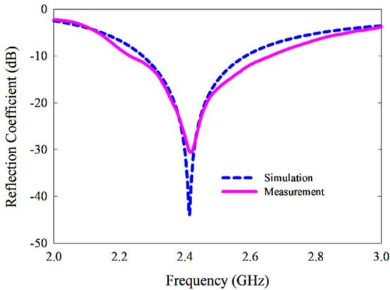
**Figure 2.** Reflection coefficient of the proposed dipole antenna without activating varactor diodes.
