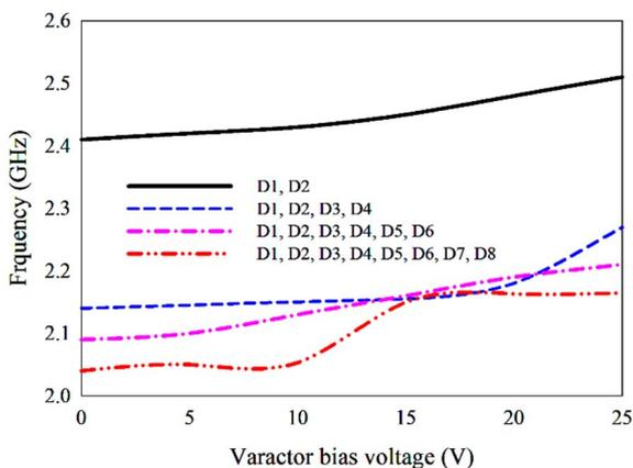
**Figure 3.** Measured variation of resonant frequency against different reverse bias voltages.
