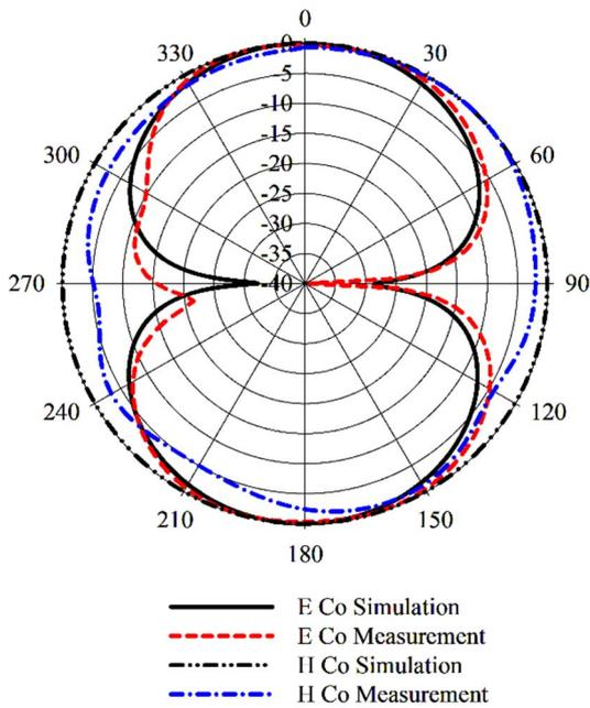
**Figure 5.** Normalized omnidirectional radiation pattern of the antenna at 2.45 GHz.
