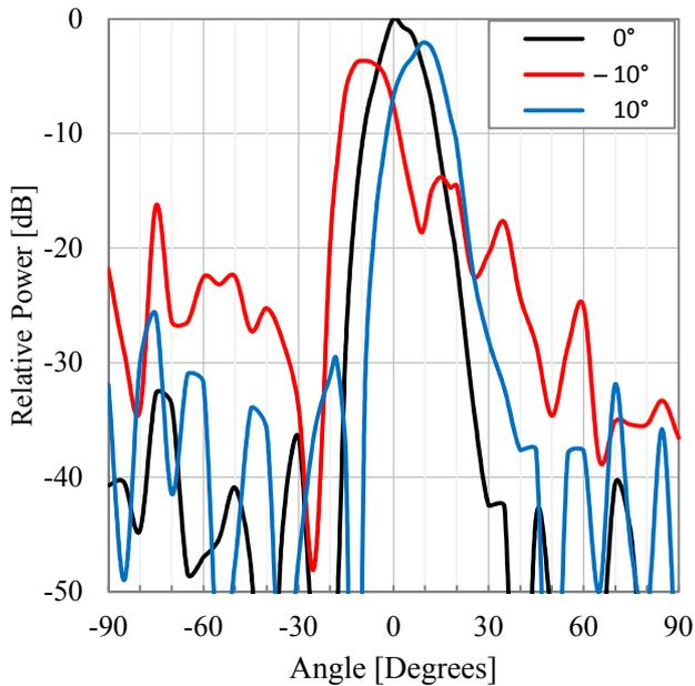
**Figure 4:** Beam-steering radiation patterns for the angles of  $0^\circ$  (black),  $-10^\circ$  (red) and  $10^\circ$  (blue) in azimuth (E-) plane.
