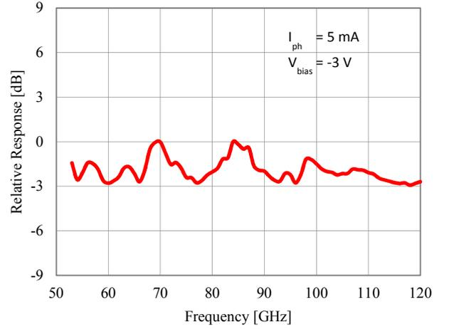
**Figure 3:** Measured frequency response of the photonic phased-array antenna emitter.
