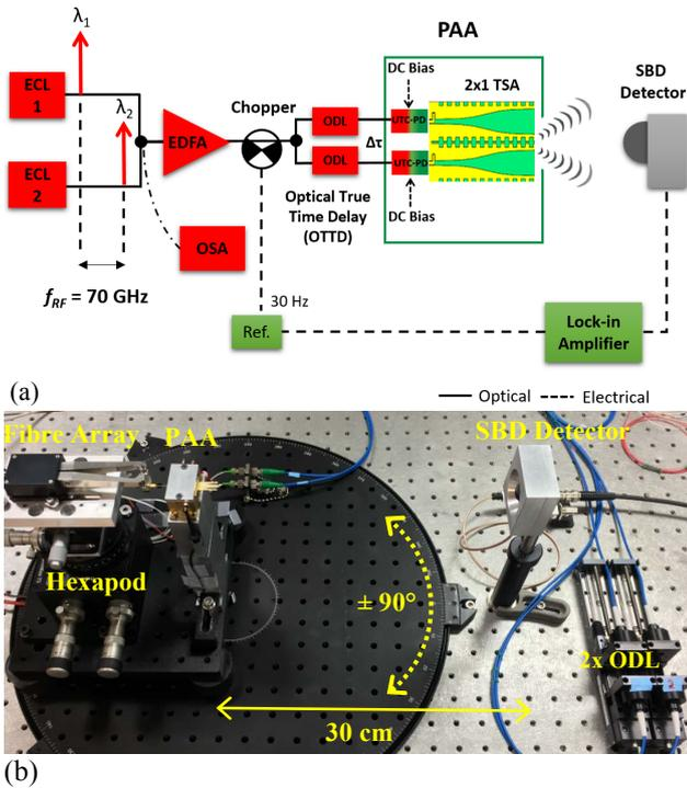
**Figure 2:** (a) Schematic diagram of the experimental arrangement for photonic-enabled beam-steering and (b) picture showing the laboratory setup for radiation pattern measurement.
