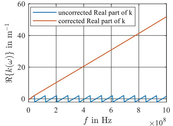
**Figure 5.** Real Part of calculated Wavenumber  $k$
