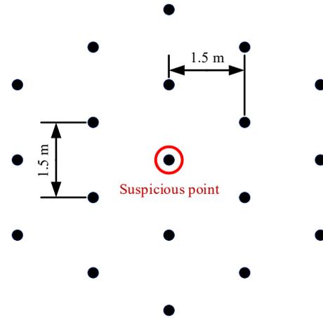
Figure 1. Example for Borehole Pattern [2]
