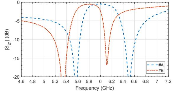
(a) Combination of filters with different bandwidth
