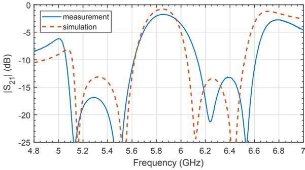
Figure 6. Comparison between the simulated and measured transmission parameters of the proposed filter.
