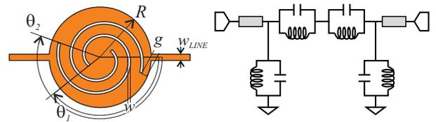
**Figure 1.** Filtering element layout and equivalent RLC circuit representation.
