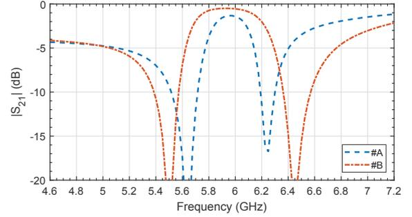
(b) Combination of filters with different center frequencies
