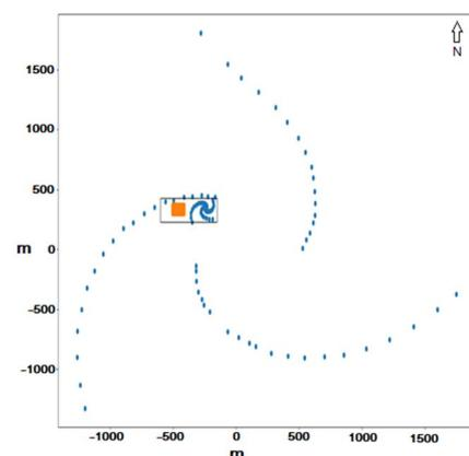
**Figure 1.** Array configuration of meter-decameter wave spectral radio heliograph. The yellow block represents the 80 LPDA calibration antennas. In the right of it are the central antennas of this array.
