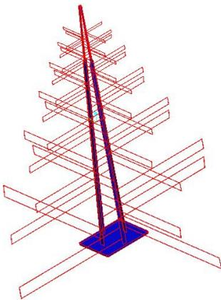
**Figure 2.** Basic design of the LPDA prototype antenna
