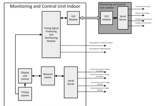
Figure 6. Interface schematic for the monitoring and control unit.
