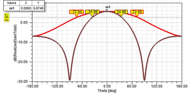
**Figure 3.** Gain patterns at 50 MHz for the prototype antenna. Red and brown lines denote H-plane and E-plane respectively.
