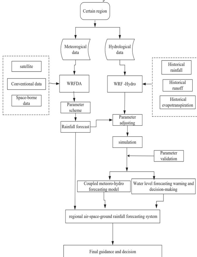
Fig. 1 Flowchart of the designed regional extreme rainfall forecasting system.
