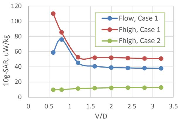
**Figure 3.** Calculated 10g-average SAR at versus the smaller axis of elliptical phantom  $V$  normalized by coil diameter  $D$  for the Cases 1 and 2.
