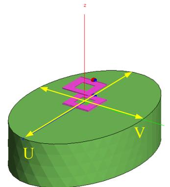
**Figure 2.** Layout of small squared spiral coils placed parallel to the elliptical phantom, Case 3.
