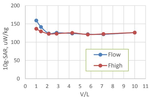
**Figure 3.** Calculated 10g-average SAR at 6.6 MHz and 7.64 MHz versus the smaller axis of elliptical phantom  $V$  normalized by squared coil diagonal  $L$  for the Case 3.
