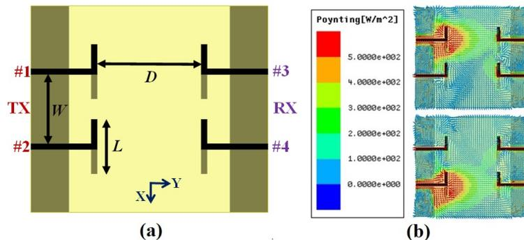
**Figure 1.** (a) Schematic diagram of a  $2 \times 2$  SR-MIMO system using printed dipoles on Arlon Substrate. Dimensions (in mm.):  $L = 29$ ,  $W = 37$  and  $D = 55$ . (b) Poynting vector distribution when either port-1 (top) or port-2 (bottom) of the Tx-end are excited at 3.5 GHz, with other ports kept in matched termination.
