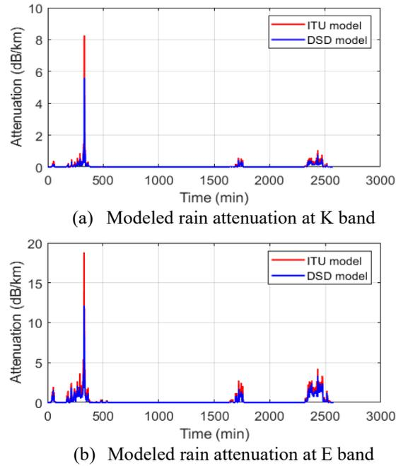
**Figure 4.** Modeled rain attenuation at K band and E band.
