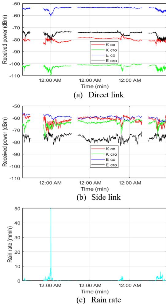
**Figure 3.** Direct and side link rain attenuations at K and E band.
