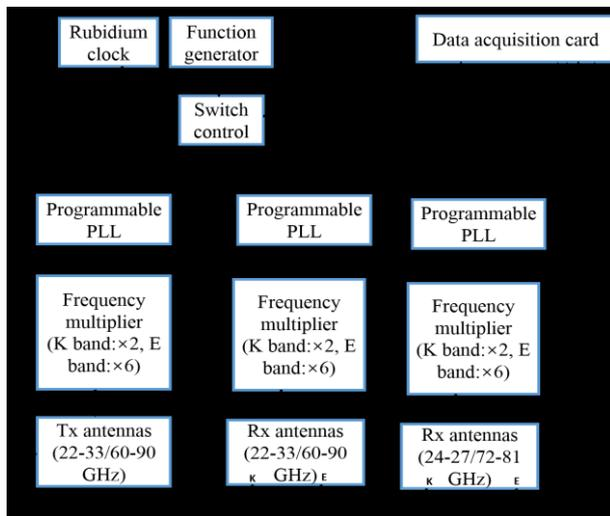
Figure 2. Block diagram of the channel sounder set up.
