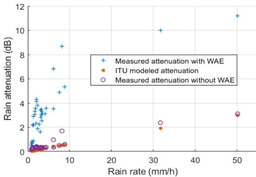
(b) Comparison of measured and estimated rain attenuations
