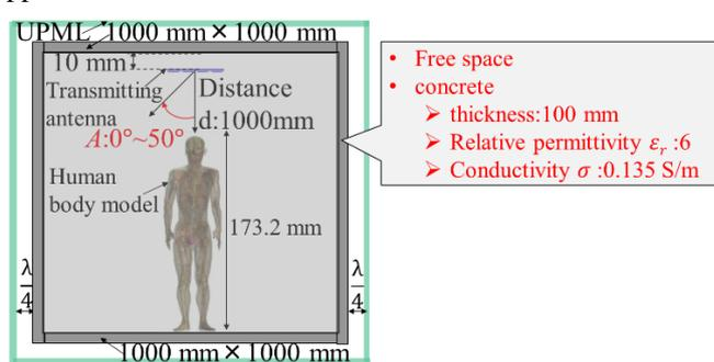
Fig. 1 Front view of simulation model.
