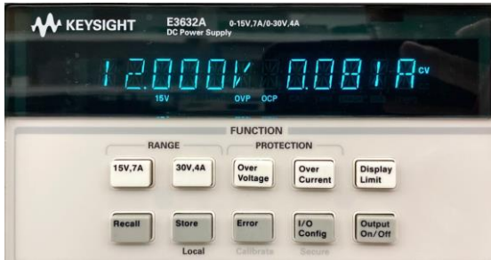
Figure 11. Input power of the entire wireless SAW generation interface electronics.
