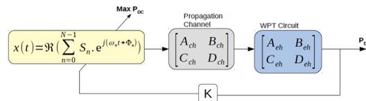
**Figure 1.** A WPT system model. The propagation channel and the rectifying circuit are modeled by their respective state-space models.
