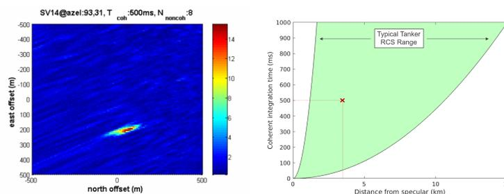
**Figure 1.** Reflection of an oil tanker (left) with detection parameters marked with "x" (right) for scenario in [2].
