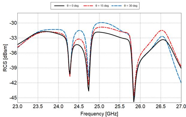
**Figure 4.** Monostatic cross-polar RCS of the tag vs. frequency for plane waves impinging from three different angles:  $0^\circ$  (continuous black),  $15^\circ$  (dash-dotted red),  $30^\circ$  (dashed blue). The spectral signature is clearly shown by three notches within the 24-26 GHz band.
