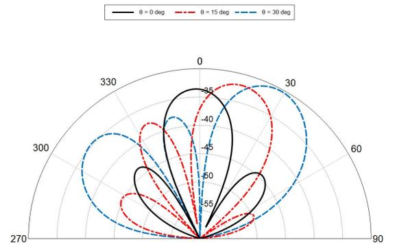
**Figure 3.** Cross-polar RCS diagrams of the tag @ 25 GHz and for plane waves impinging from three different angles:  $0^\circ$  (continuous black),  $15^\circ$  (dash-dotted red),  $30^\circ$  (dashed blue).
