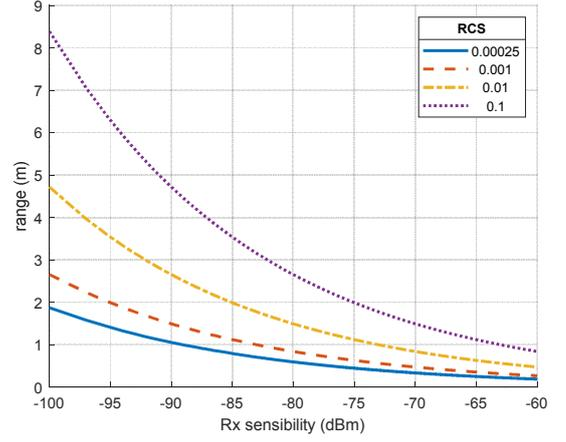
**Figure 1.** Lossless radar range @ 24 GHz vs. receiver sensibility for different values of tag's RCS, 8 dBm transmitting power with 5 dB antenna's gain.
