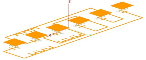
**Figure 2.** 3D layout of the tag antenna with dielectric layers and ground planes removed. The visible parts are: patches, slots and network that lie on three different layers. U-shaped resonators are also visible.
