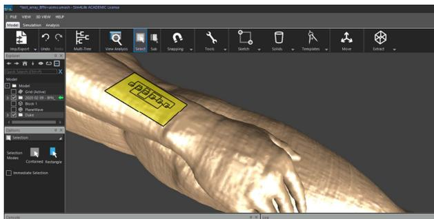
**Figure 5.** FDTD model of the proposed chipless tag, when positioned on a portion of a human forearm. Analyzed by *Sim4Life* simulation platform [11].
