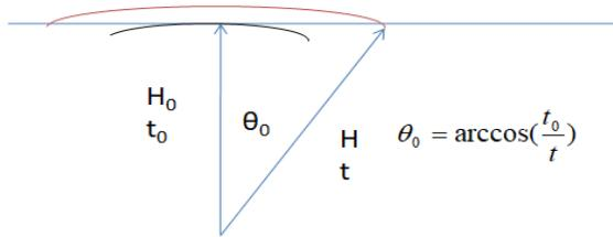
**Figure 3.** Measurement scheme of an acoustic wave gauge.
