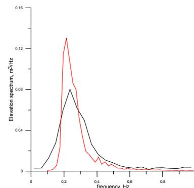
Figure 2. Sea surface waves spectrum measurements. The black line – acoustic wave gauge, the red line – string wave gauge.
