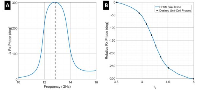
**Figure 4.** (a) Simulated tunable phase range of the CID-SP over frequency. A maximum phased tuning range of  $301^\circ$  degrees is achieved at 12.8 GHz (denoted by black dashed line). (b) Simulated Rx phase over the tunable permittivity ( $\epsilon_r$ ) for the BST material. The black diamonds denote the  $\epsilon_r$  values shown in Table 1 that realize an equally-spaced progressive phase shift for radiation pattern scanning.
