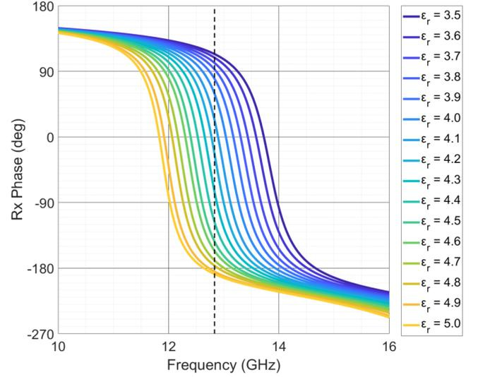
**Figure 3.** Simulated reflection (Rx) phase using HFSS for the CID-SP unit-cell over frequency for different  $\epsilon_r$  values within the tunable range of the BST material substrate. The vertical dashed line denotes the operating frequency of 12.8 GHz, which provides the maximum  $301^\circ$  degrees of Rx phase tunability for the CID-SP.
