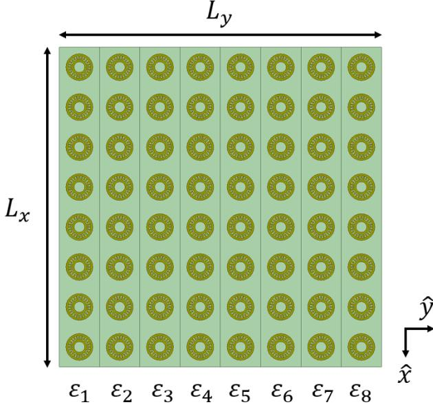
**Figure 1.** The proposed MTS composes of 8-by-8 circular inter-digitated self-phased (CID-SP) cells. Each column has an independently tunable BST substrate permittivity  $\epsilon_r$ . By changing the by a bias voltage applied to the BST, the desired reflection (Rx) phase can be achieved. The dimensions of the 8-by-8 are  $L_x = L_y = 48$  mm. The height of the R-MTS is  $h = 1$  mm, which is  $\lambda_0/23.4$  at the operating frequency of  $f_0 = 12.8$  GHz
