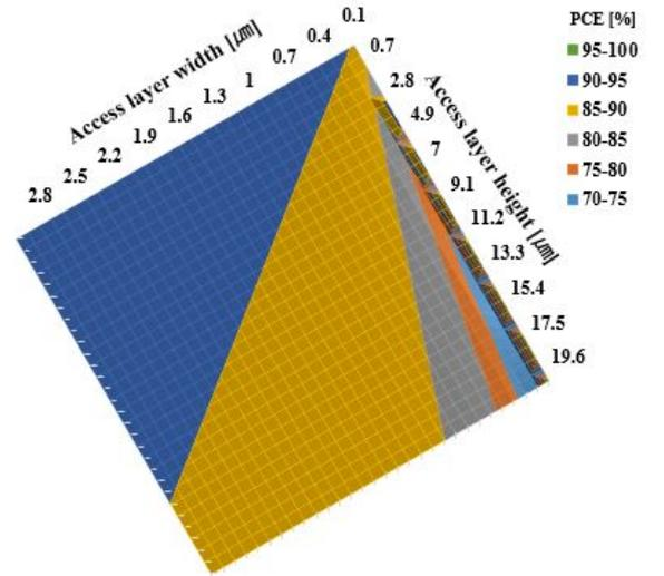
**Fig. 2.** GaN Schottky diode structure and energy-conversion efficiency when Access layer width and height varied with  $V_{out}=40\text{V}$ ,  $C_{j0}=0.325\text{pF}$ ,  $V_{bi}=0.912\text{V}$ ,  $R_L=150\Omega$ ,  $r=50\Omega$  and  $\alpha=0.3$ .
