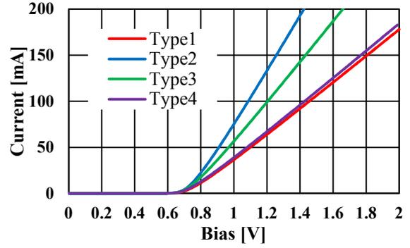
**Fig. 3.** I-V characteristics of diodes.
