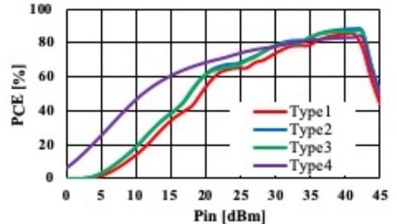
**Fig. 5.**Power-conversion efficiency of high efficiency rectifier with  $330\ \Omega$  load resistance.
