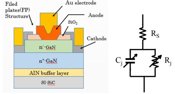
**Fig. 1.** Structure of GaN Schottky diode and equivalent circuit
