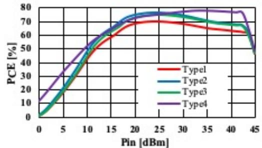
Fig. 6. Power-conversion efficiency of wide dynamic range rectifier with 330  $\Omega$  load resistance.
