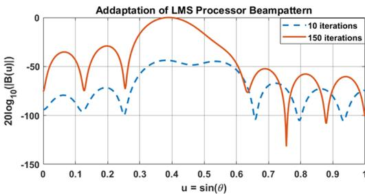
**Figure 1.** The adaptation of the LMS processor beam pattern. The desired signal is located at  $u = 0.382$  while the interference signal location is  $u = 0.886$ .
