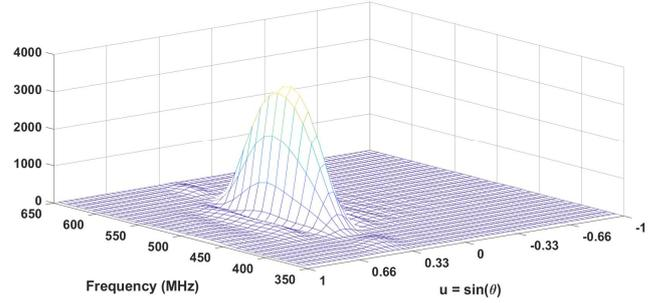
**Figure 2** The space-time response beam of the wideband LMS processor. The desired signal is located at  $u = 0.5$  and has a center frequency 500 MHz.
